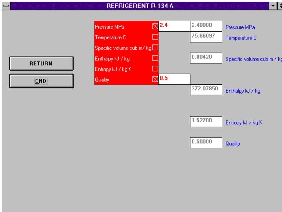
Figure 2 Fluid Properties with Two Conditions Specified
