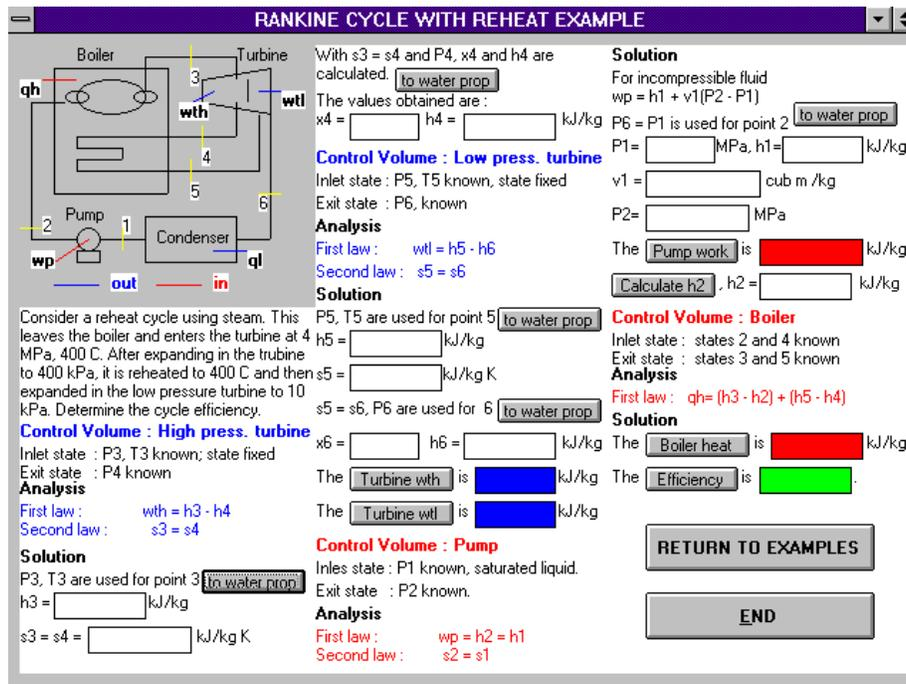
Figure 4 Example on Rankine Cycle with Reheat
