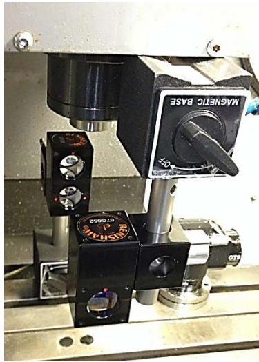
Figure 3 Renishaw Laser XL Angular Measurement System mounted
