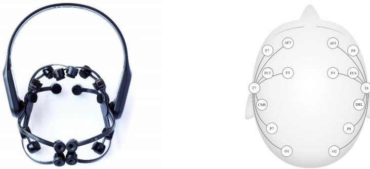
Fig. 2. EPOC X EEG headset and the position of the EEG electrodes on the scalp [7].
