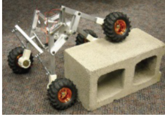
Figure 8. The rear linkage set, adding stability by relating the movement of the right and left linkage chains
