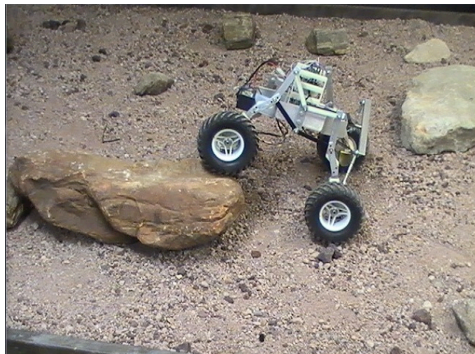
Figure 11. Testing the rover platform on “Planet Mars” environment
