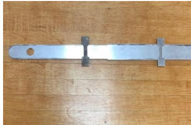
Figure 2 – Fabricated plate to hold the heating rod (through the hole) and fit into the wind tunnel
