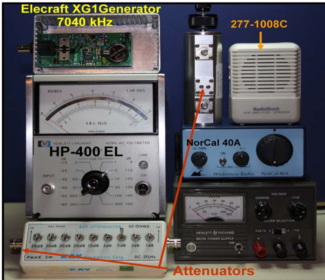
Figure 6: CW Minimum Discernable Signal Equipment used in Test-Setup
