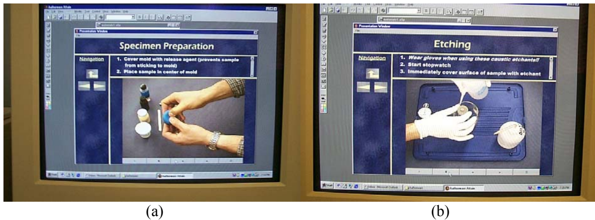
Figure 1. The metallography experiment showing various preparation stages of the sample: a) mounting and b) etching.
