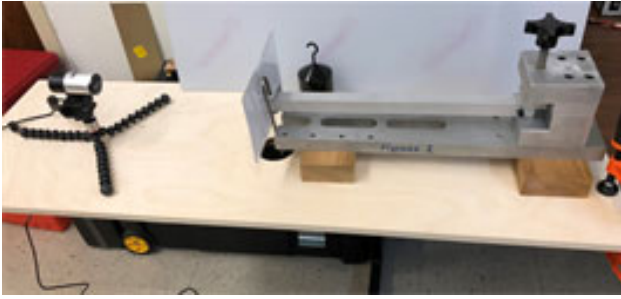
(a) Setup on wooden platform cantilevered over table edge and ready to test using kg weight attached to tip behind the target
