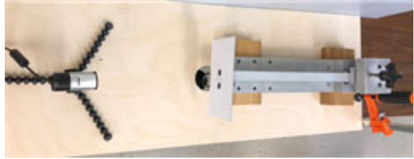
(b) View of test setup from overhead showing webcam aimed at tip target
