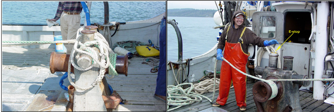
A capstan -type winch with fishing lines wound around.
