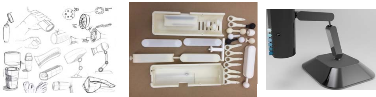
Figure 4: Concept sketches, 3D prints, and a rendered image of the proposed solution, Team 4, multispectral USB microscope
