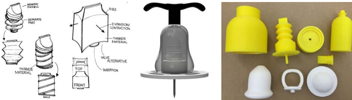
Figure A1: Example concept sketches, rendered image, and 3D prints produced by team 1, neonatal pneumothorax
