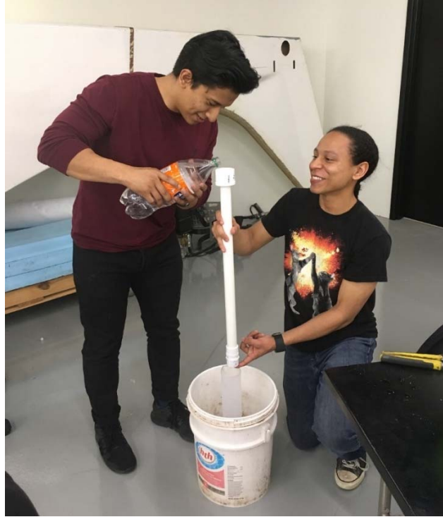
Figure 10 Student on right holding tube with right hand and with finger over opening with the left hand. Student on the left maintaining water level with old soda bottle filled with water. A graduated cylinder is inside the bucket.
