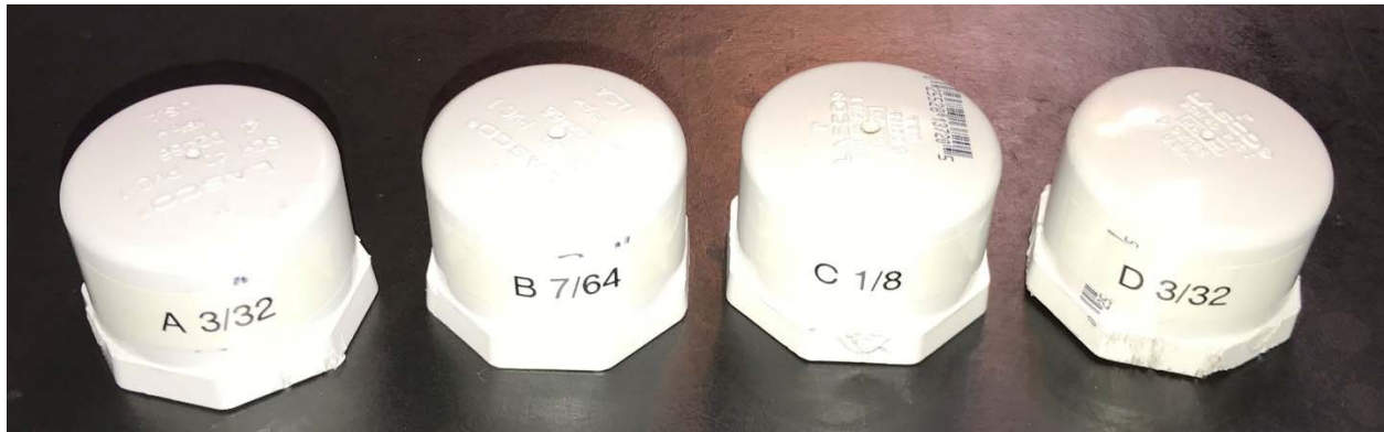
Figure 5. Caps used for experiments made of 1" PVC.
