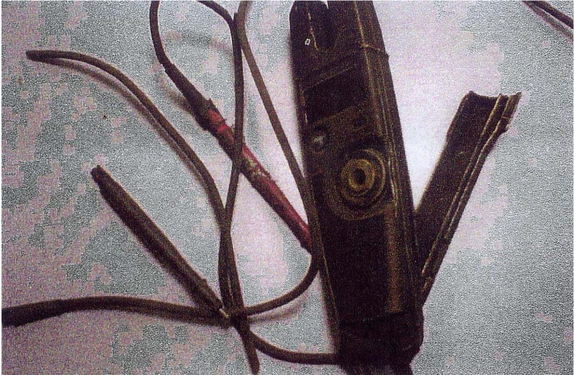
Figure 3: Bright yellow fluke multi-meter is badly blackened (burnt) out a result of measuring 4000 Volts.
