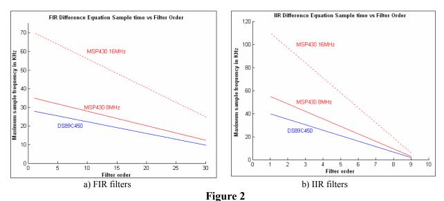
Maximum sample frequency vs. filter order for a) FIR filters and b) IIR filters. This is an exploded scale view of Figure 1 with the much faster ARM 7 processor omitted.
