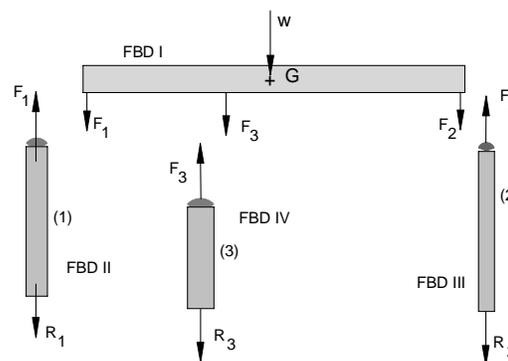
Figure A.2. Beam and posts free body diagrams.
