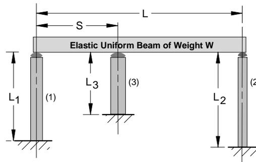
Figure A.1. Statically indeterminate elastic beam supported by elastic posts.
