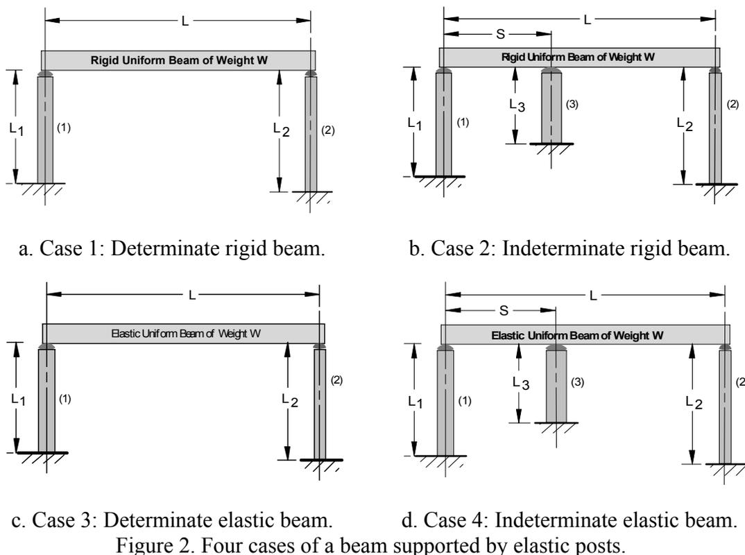
Figure 2. Four cases of a beam supported by elastic posts.
