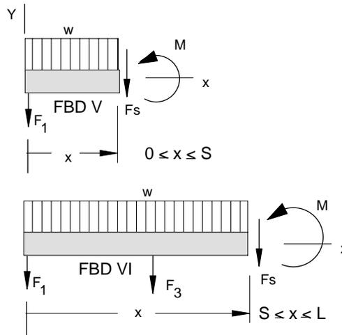
Figure A.4. Beam free body diagrams.
