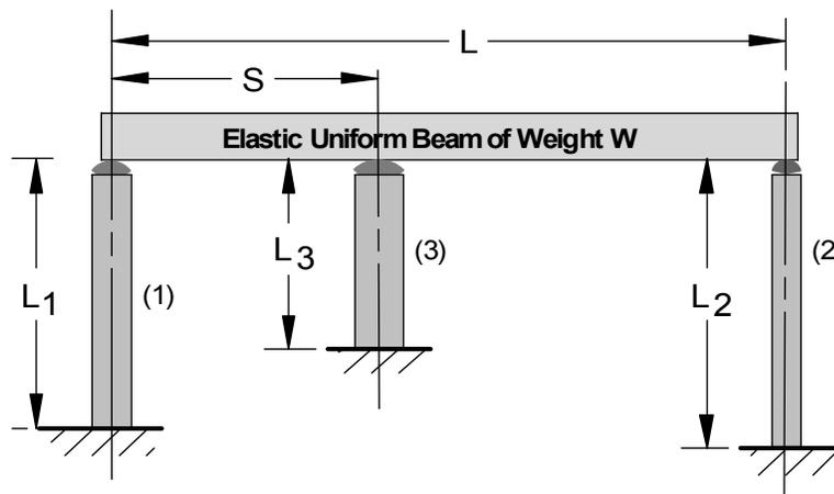
Figure 1. Statically indeterminate elastic beam supported by elastic posts.
