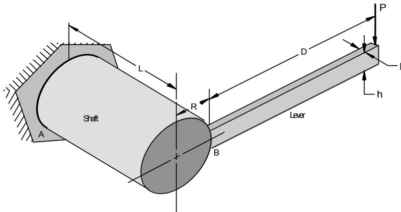
Figure 3. Cantilever circular elastic shaft with an attached elastic lever.
