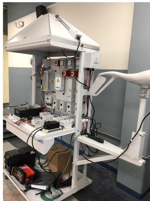
Photo 1b. Solar/Wind Energy Training System
