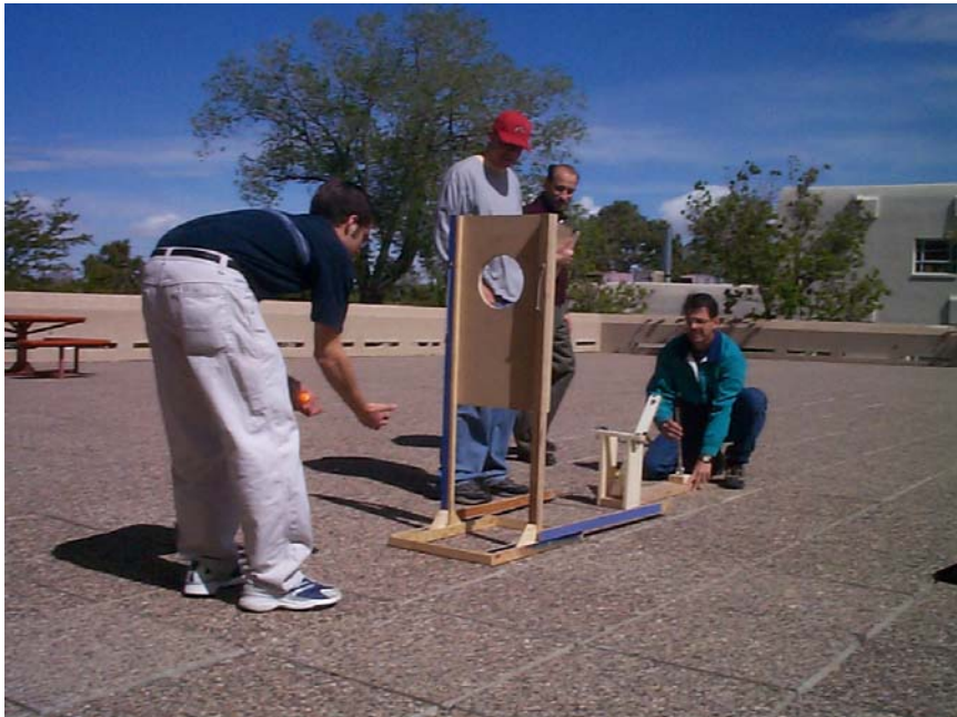
Figure 4. A design utilizing an elastic rubber band to catapult a golf ball. Before launch, the ball was seated in a smaller size hole at the end of the swinging catapult arm. Notice the student on the left-hand side catching the ball with his left hand (the ball is colored orange in this case).
