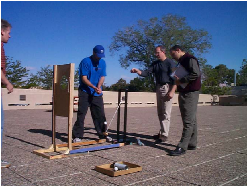
Figure 3. A design that relied on the impact of a pendulum with the golf ball in order to shoot it in the air. In this picture, the pendulum (composed of a chamfered metallic solid cylinder attached to a rigid rod) is shown after it just hit the golf ball.
