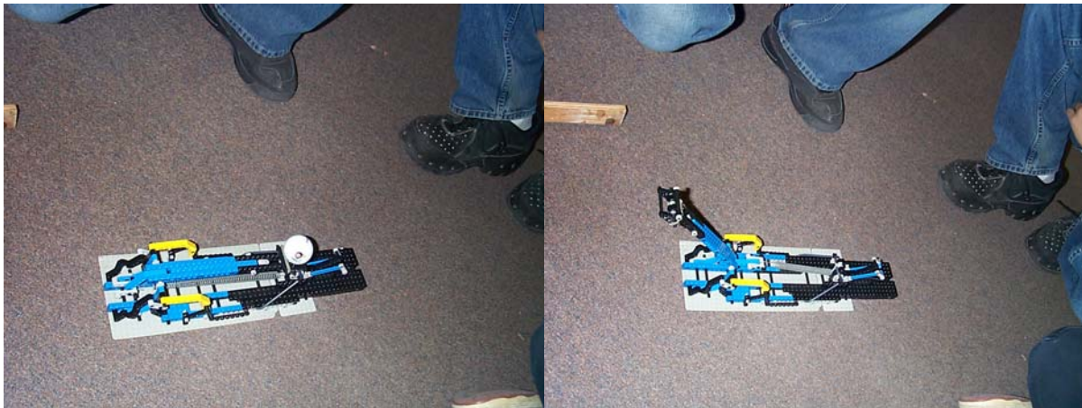
Figure 6. (a) The golf ball shown ready for launch from the LEGO catapult. (b) The catapult shown in the released configuration. The release energy comes off of a stretched spring placed underneath the catapult arm.
