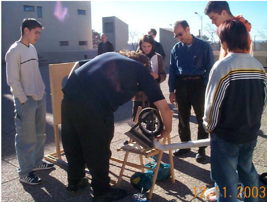
Figure 7. A design utilizing a motor-driven wheel to accelerate a golf ball through a tube shoot.
