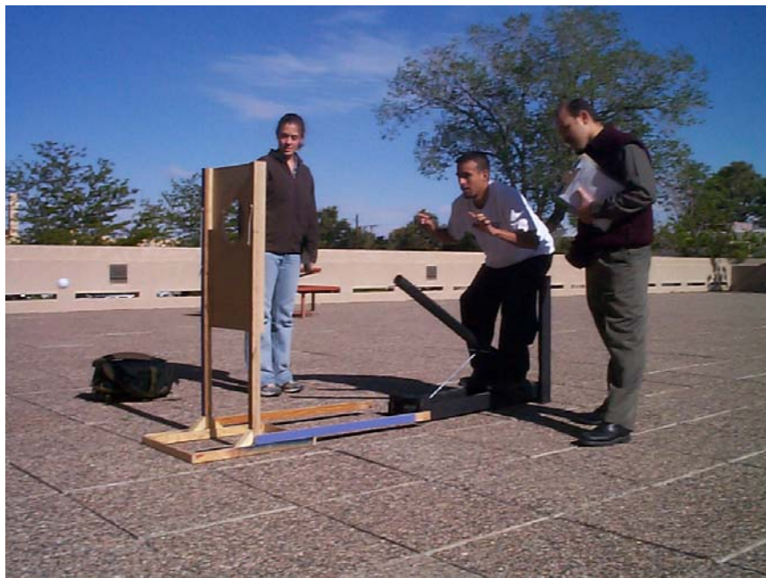
Figure 2. A design utilizing a compression spring tilted at an angle from the floor. The spring was enclosed inside a plastic tube.
