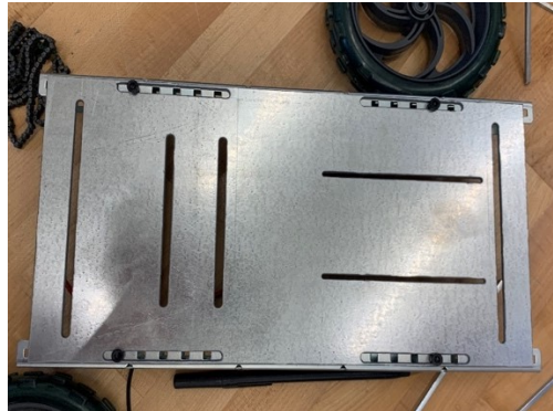
Figure 2: Chassis made with Water Jet in Implementation Phase
