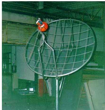
Figure 2. Offset parabolic reflector built and tested for satellite TV reception at C-band.
