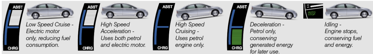
Figure 1. Energy sources in a typical HEV subject to driving conditions [15]
