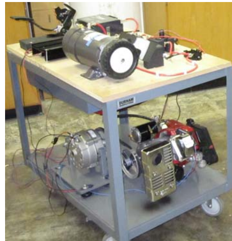
Series electric-drive portion on the bottom of the cart
