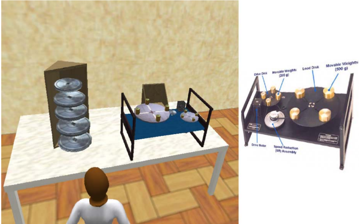
Figure 4: Industrial plant emulator (right) and its virtual model in OpenSimulator (left)
