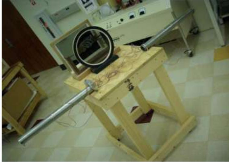
Figure 4 . Open and closed tube test setup for application of torsion and bending
