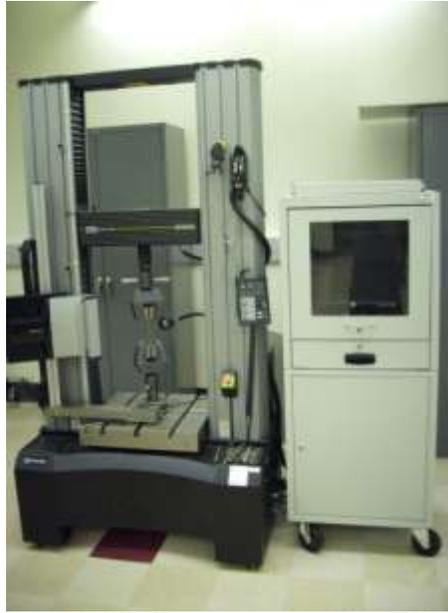
Figure 9. Instron universal testing machine model 5882
