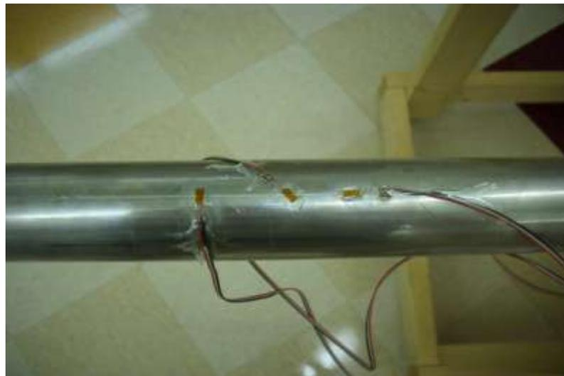
Figure 5. The three strain gauge sensors orientated at 0°, 45°, and 90°
