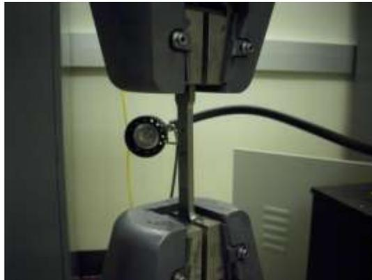
Figure 10. ASTM sample placed in the jaws of the Instron machine for tensile testing
