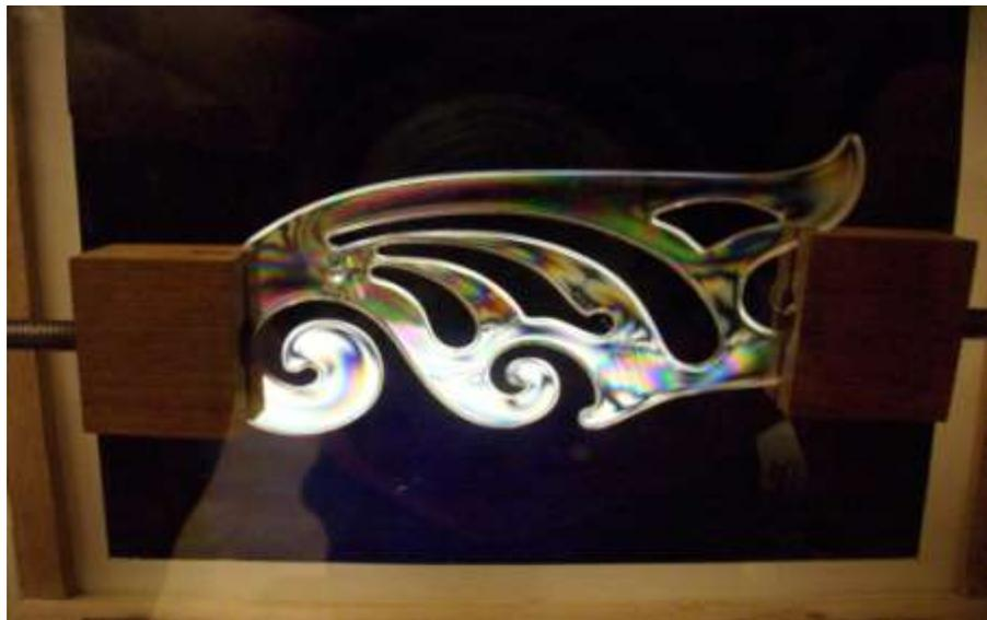
Figure 1. Residual stress patterns displayed by polarized light in a French curve
