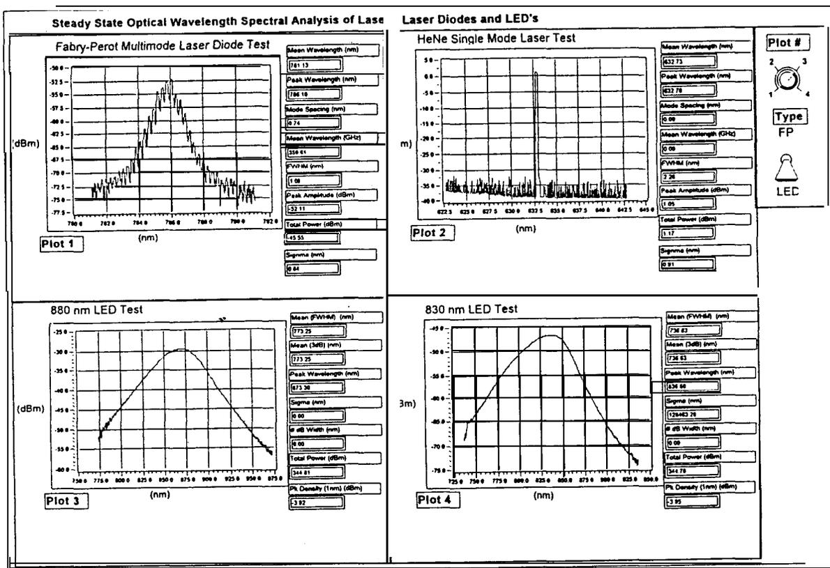
Figure 4: Power spectra of optical sources (1) 780 nm Fabry-Perot laser spectrum, (2) 633 nm He-Ne laser spectrum, (3) 880 nm LED spectrum, (4) 830 nm LED spectrum.
