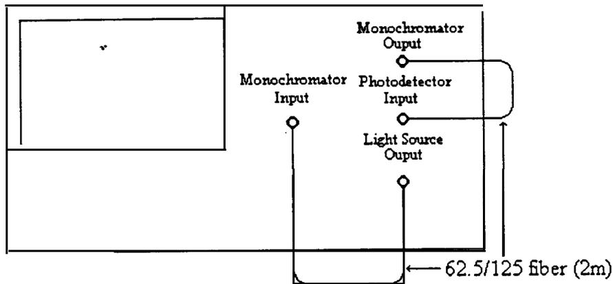
Setup for measuring responsivity of a photodiode
