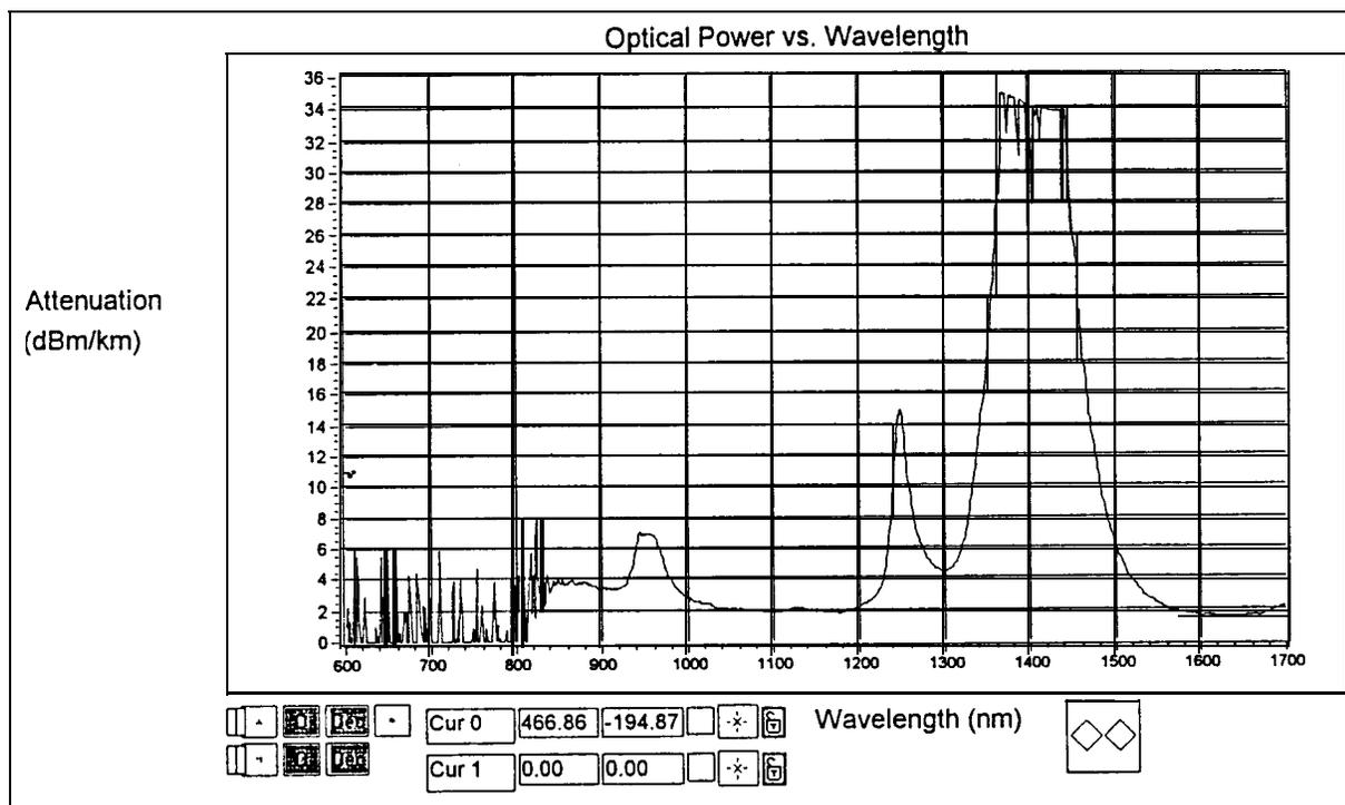
Figure 2: Measured spectral attenuation for a 100/140 mm GRIN fiber.
