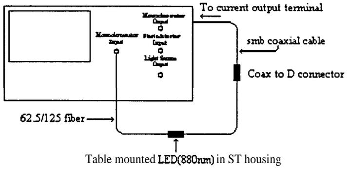
Figure 3: Experimental measurement of laser and LED spectra.
