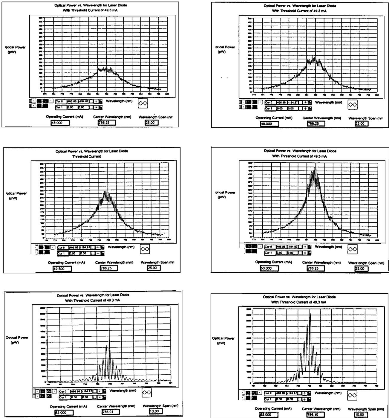
Figure 5: Dynamic changes in a Fabry-Perot laser diode spectra in the vicinity of the threshold current showing samples of the spectra at different drive currents.
