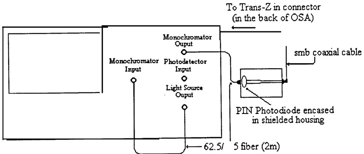
Figure 6: Measurement of spectral responsivity of photodiodes.
