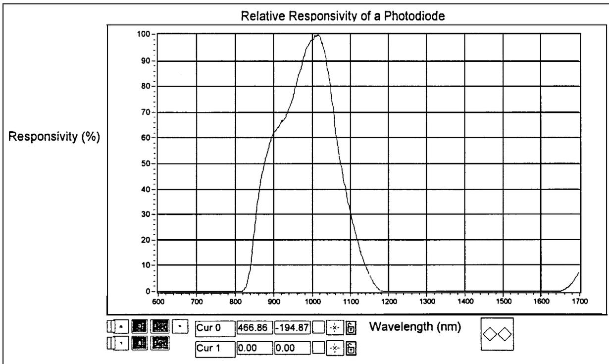
Figure 7: Spectral responsivity of a PIN photodiode.
