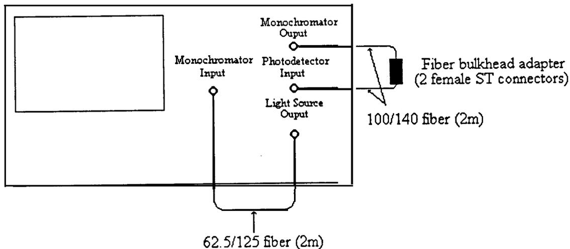
Figure 1a: Measurement of fiber spectral attenuation.
