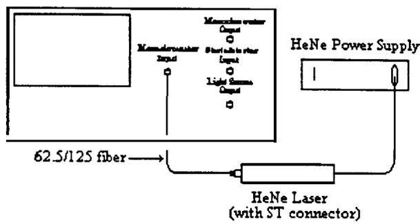
Setup for measuring 880nm LED
