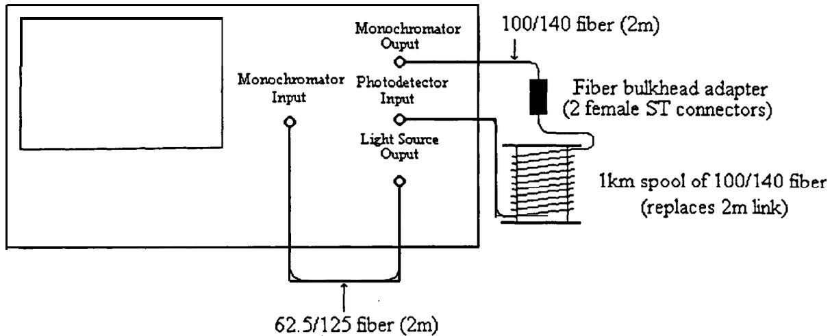
Figure 1b: Measurement of fiber spectral attenuation.
