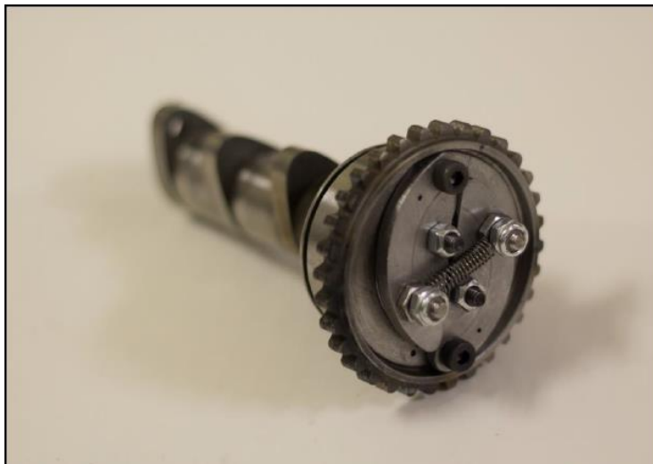
Figure 2: An example of a prototype built in the capstone design program: a cam phaser
