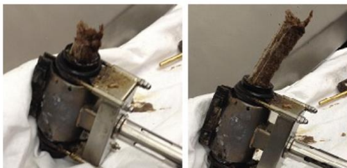
Figure 4: Rapid Expansion of composite material due to moisture content [3]
