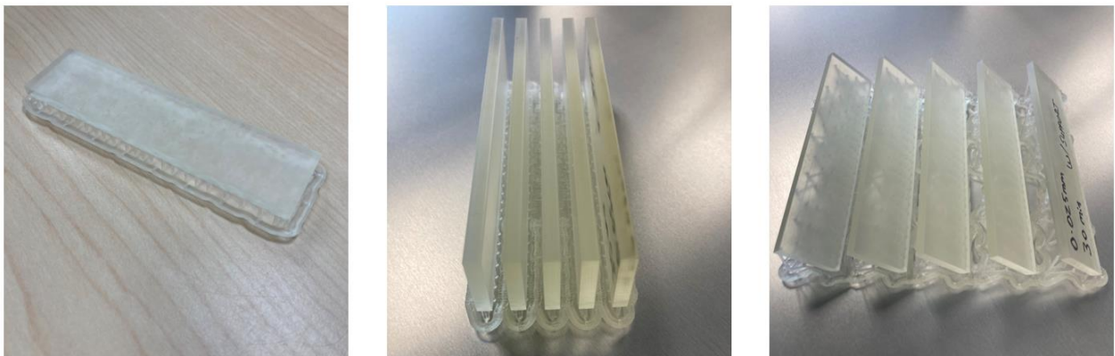
Figure 2. Samples printed at 0° (on the left), 45° (in the right), and 90° (in the middle)
