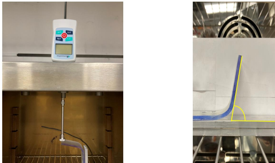
Figure 6. Test setups for shape recovery force (on the left) and shape recovery speed (on the right)
