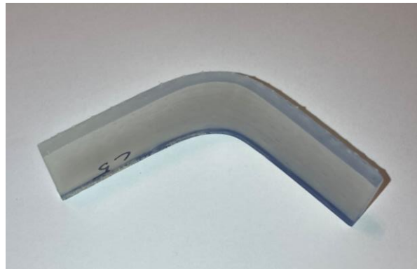
Figure 3. Programmed part with 90^\circ bend.
