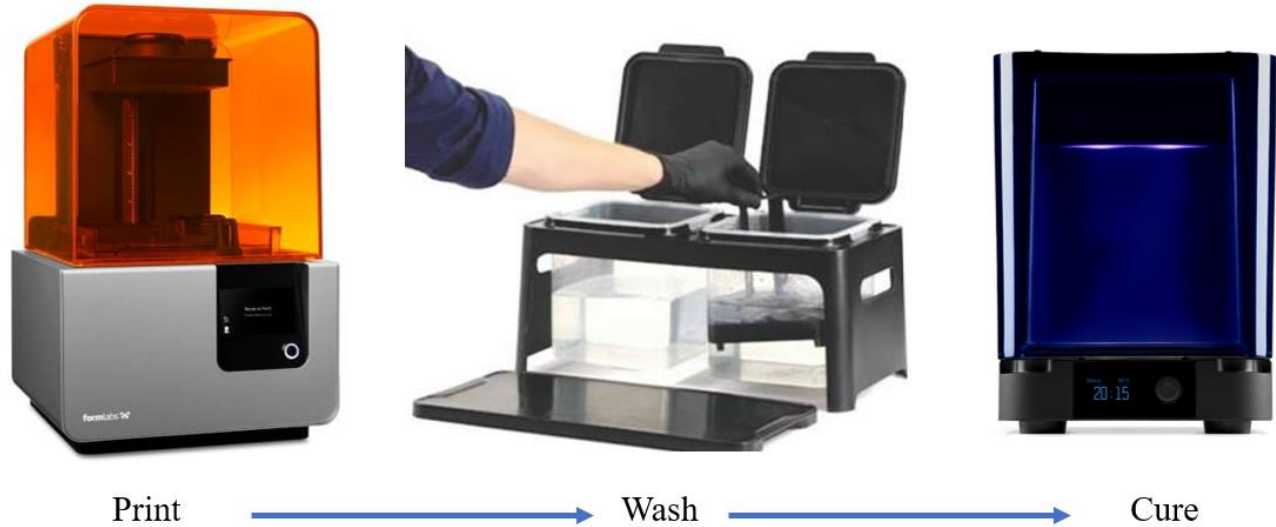
Figure 1. Formlabs Form 2 (on the left) wash tank (in the middle) and Form Cure (on the right)
