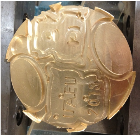
Figure 4: Nested parts inside the Shaft (Before Parting off)
