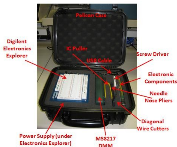
Figure 2: Portable electronics self-contained lab components including the EEBoard.
