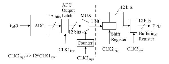
Figure 1: A High-Speed Data Transfer and Buffering Scheme for Input Capture
