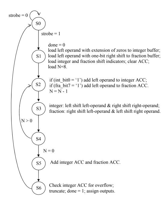
Figure 6: Control Flow of A Multiplier
