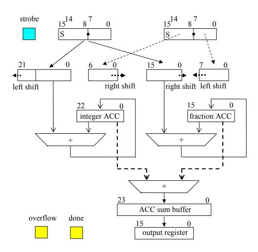
Figure 5: Data Paths of A Sequential Multiplier
