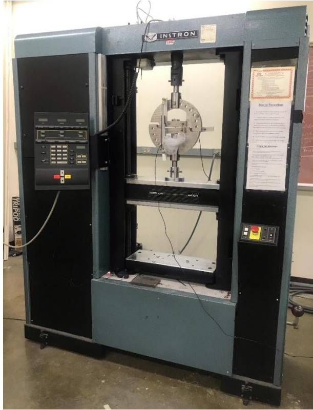
Figure 1: An Instron 4400R Load Frame for Tension/Compression
