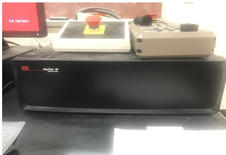
Figure 3. MTS FlexTest 40 controller used to record load-displacement and LVDT data
