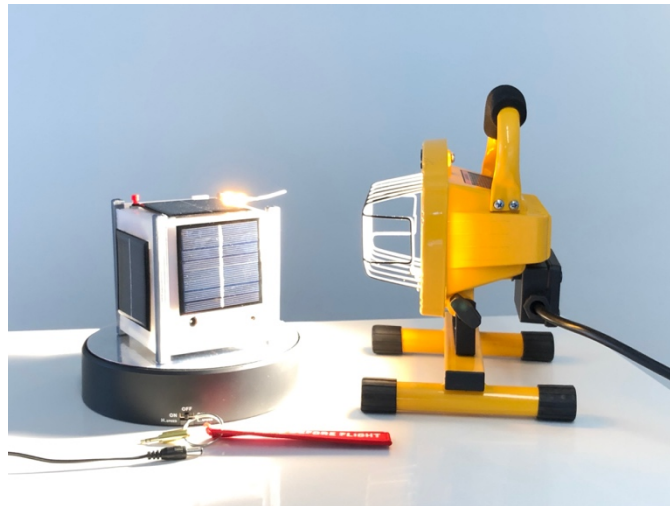
Fig. 1. AMSAT CubeSat Simulator on a rotating turntable in front of a halogen lamp to simulate rotation on orbit.
