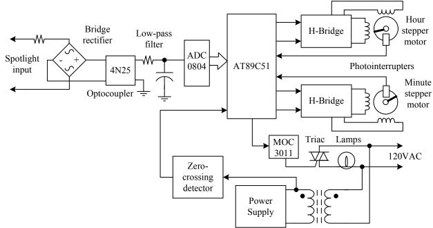
Fig. 4. Block diagram of the microprocessor-controlled grandfather clock
