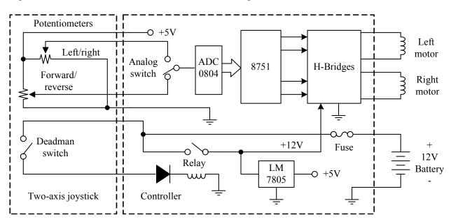
Figure 3 shows the motorization scheme in block-diagram form.
