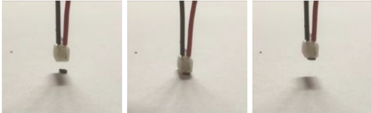
Fig. 13: b-1.0-0.5-1.0-5.0 type device picking up a sesame seed
