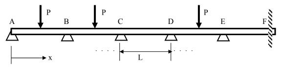
$M_{max}$  is found from a moment diagram followed by  $M_{all} = M_{max} / F.S. = \sigma_{all} S$ , where  $\sigma_{all} = \sigma_{ULT} / F.S.$ ; and S is the elastic section modulus. This problem would not be routinely assigned to sophomores for homework.
