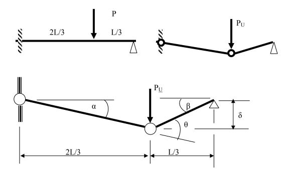
Angles  $\alpha$ ,  $\beta$ ,  $\theta$  and deflection  $\delta$  are used in connection with L to describe the collapse geometry.
