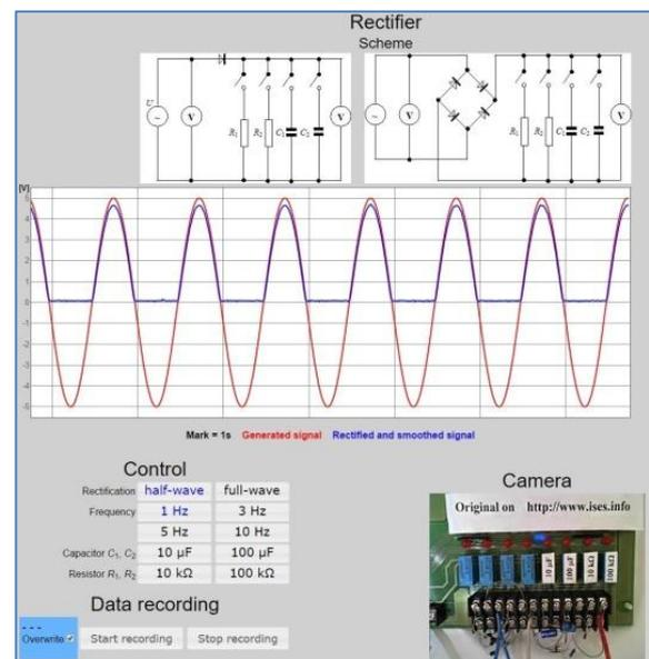
**Figure 2** Alternating Current Rectifier
