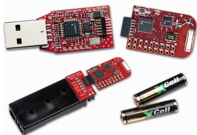
Fig. 10b: TI eZ430-RF2500 development kit 6
