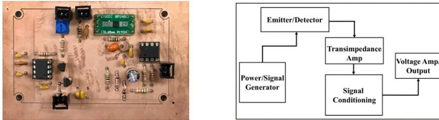
Figure 2: Spectrophotometer circuit designed and constructed at Norwich. Key subsystems/functions of the circuit (right) are shown alongside the physical board (left).
