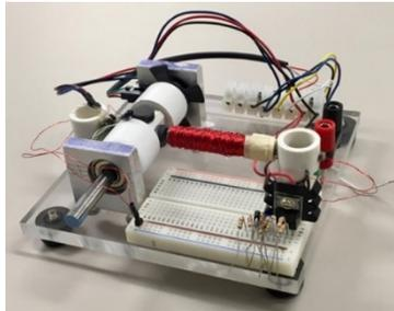
Figure 1: BLDC kit used for Lab 3. This is a modified Simple Motors kit [7]; the modifications include: reinforced, threaded mounts, a rotor mechanism including a robust steel axle/roller skate bearing assembly, and DC power supply ports to combat current supply issues with the batteries.
