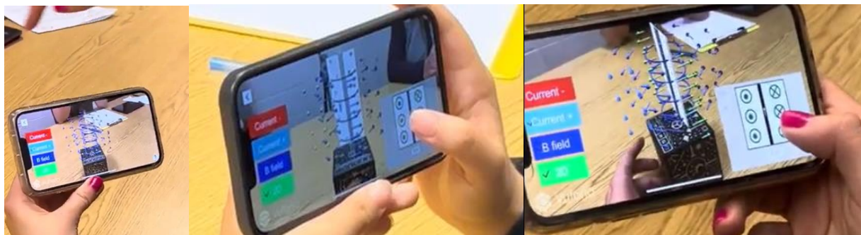
Fig 4. (a) The MARVLS simulation exploring the relationship between electric current and magnetic fields, (b) screenshot of the simulation with the 3D and 2D representations, (c) when the user touches the 2D representation, the arrows on the 2D plane are highlighted.
