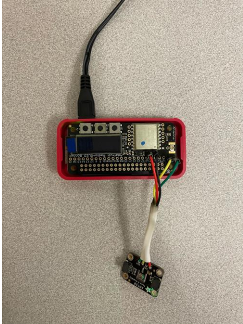
Figure 3.1: CS connected with I2C Sensor
