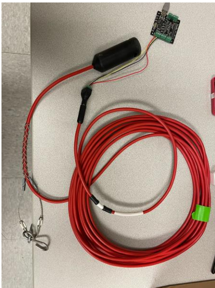
Figure 3.3: Hydos Water sensor connected to SDI-12 External board with 3-Channel audio input to USB
