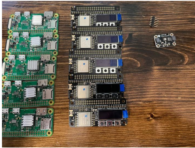
Figure 3.0: Raspberry Pi 0 and Adafruit LoRa Radio Bonnets (separated for example)
