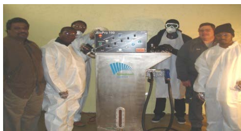
Figure 4a. BioPro 190 at the UMES Biodiesel facility for making biodiesel from waste cooking oil
