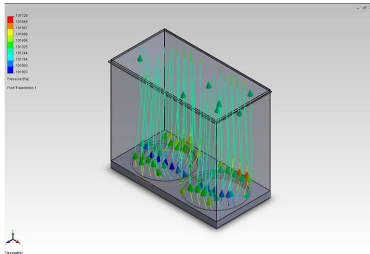
Figure 12. Initial flow simulation model (fan swirl 2rad/s).
