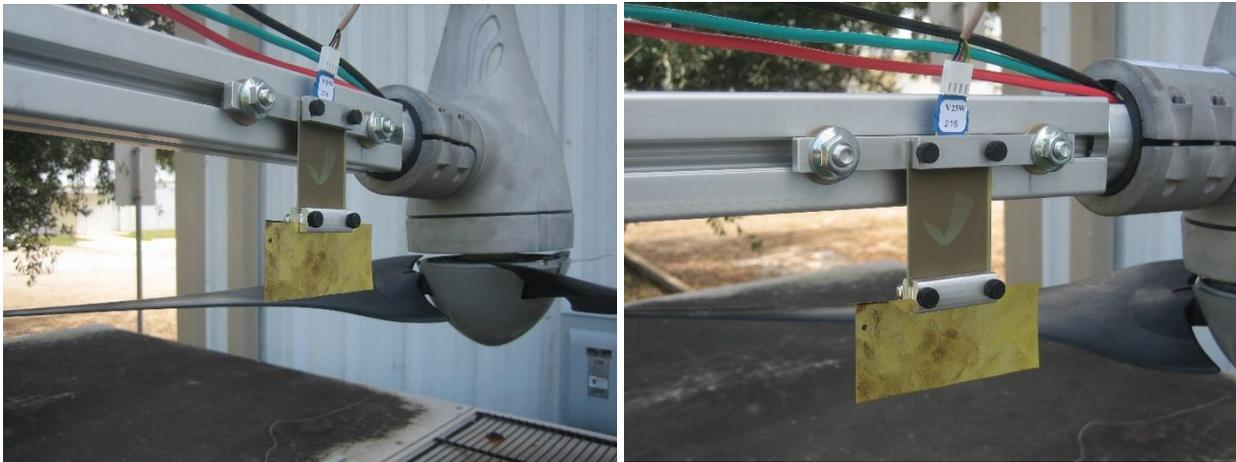
Figure 13. Mide vulture piezoelectric device under testing – mounted to wind turbine stand
