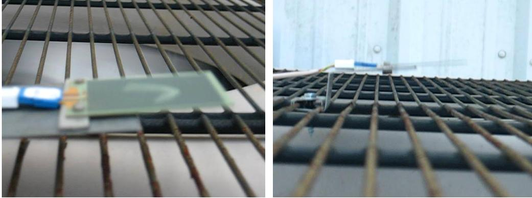
Figure 14. Mid voltage piezoelectric device under testing – *mounted to exhaust grid*
