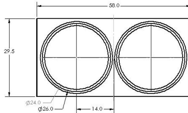
Figure 5. Fan housing dimensions (top view, inches)
