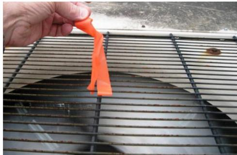
Figure 10. Tape held at center of fan showing vacuum.
