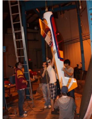
Figure 1: Swing Tests for Measuring Aircraft Moment of Inertia
