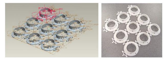
Figure 3: Astroturf structural membranes: CAD model, rapid prototype
