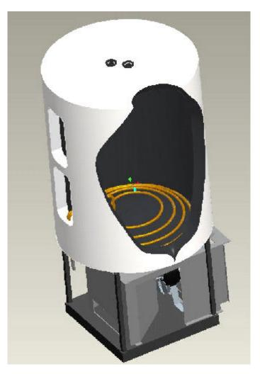
Figure 1: Hybrid Water Heater and Dehumidifier
