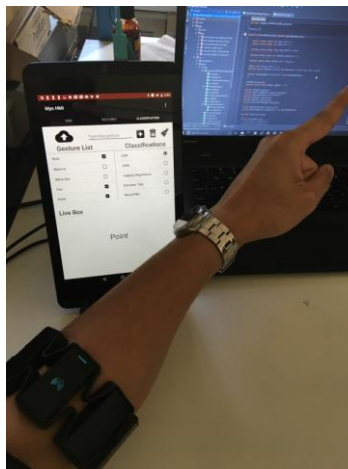
Figure 4. The Android application predicting the subject's current gesture (point) in real time.
