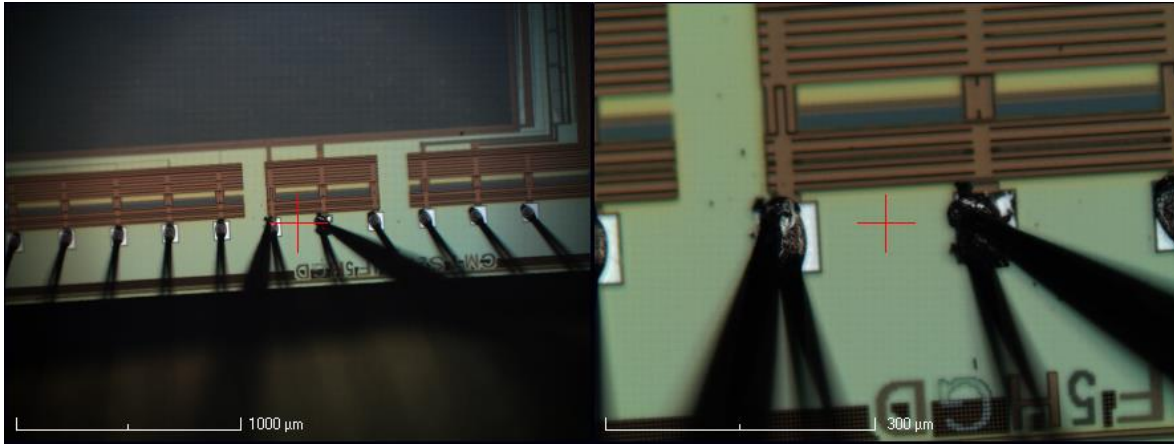
Figure 18. Power supply section of chip under test
