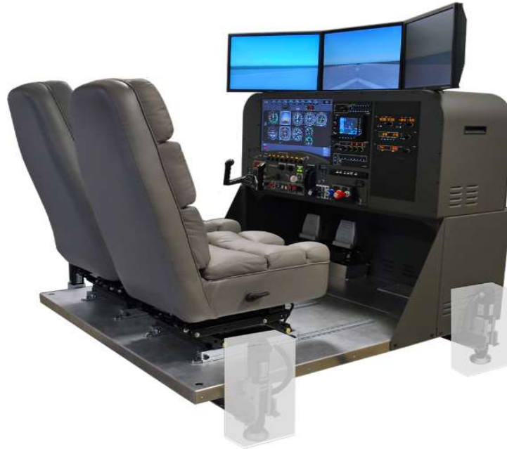
Figure 2: Flight Training Device (FTD) - aka Flight Simulator
