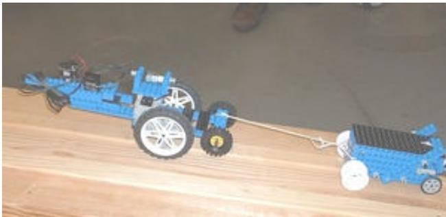
**Figure 1:** Motorized Cart Pulling Load up Incline
