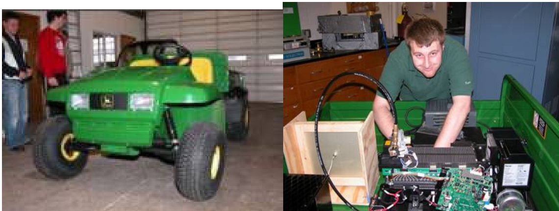
Figure 3. John Deere e-Gator with fuel cell power unit as the payload.
