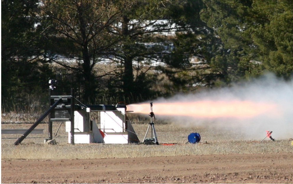
Figure 2: Rocket Motor Static-Fire Test
