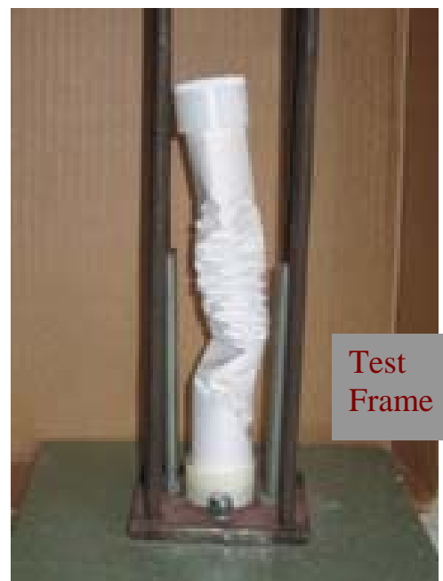
Paper Column, After Buckling Figure-8
