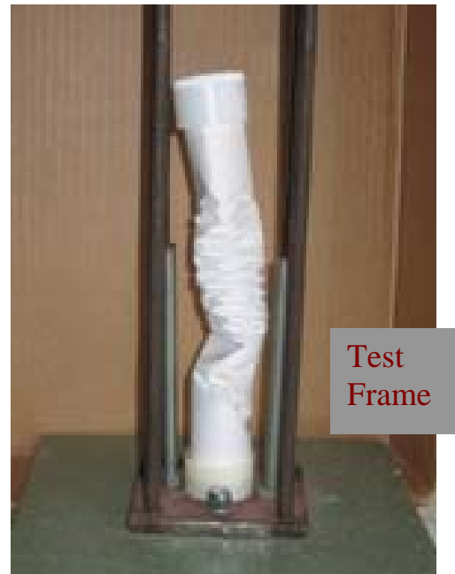
Paper Column, After Buckling Figure-8
